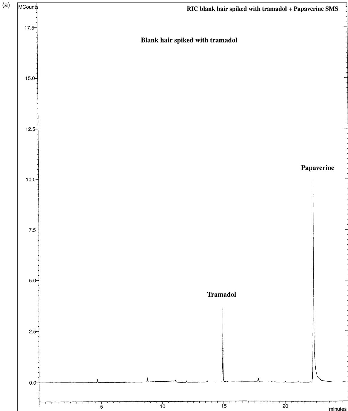
Fig. 1. The GC-MS/SIS chromatograms of: (a) blank hair spiked with tramadol hair; (b) blank hair and (c) hair sample taken from case no. 1.
